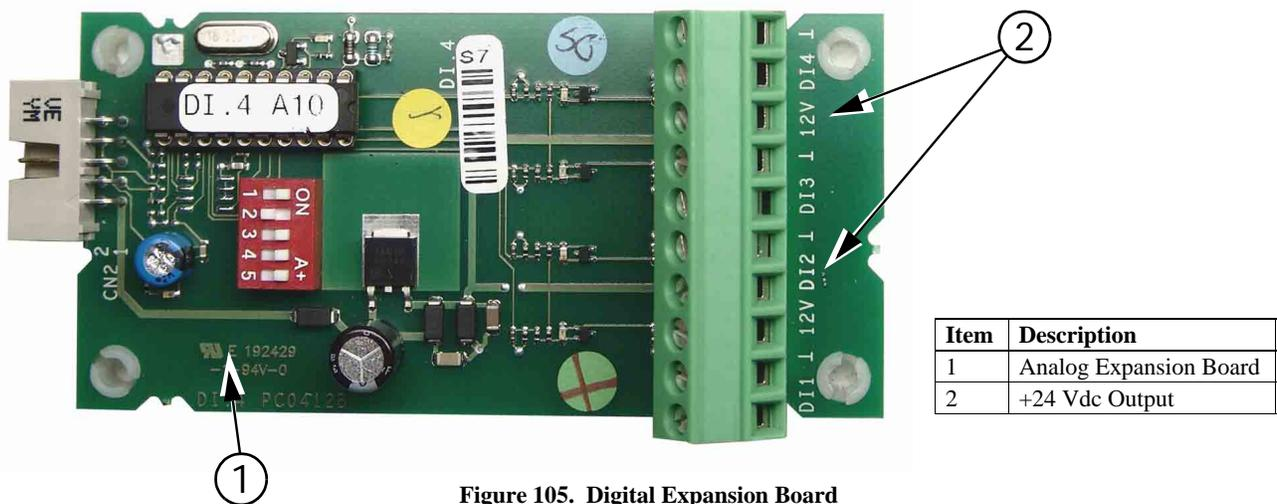
Figure 105. Digital Expansion Board
