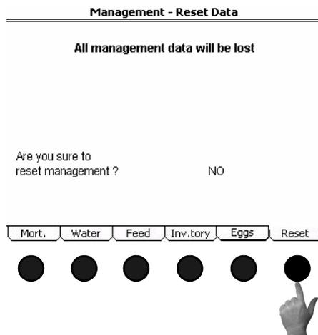
**Figure 52. Management Screen: Reset Tab**
