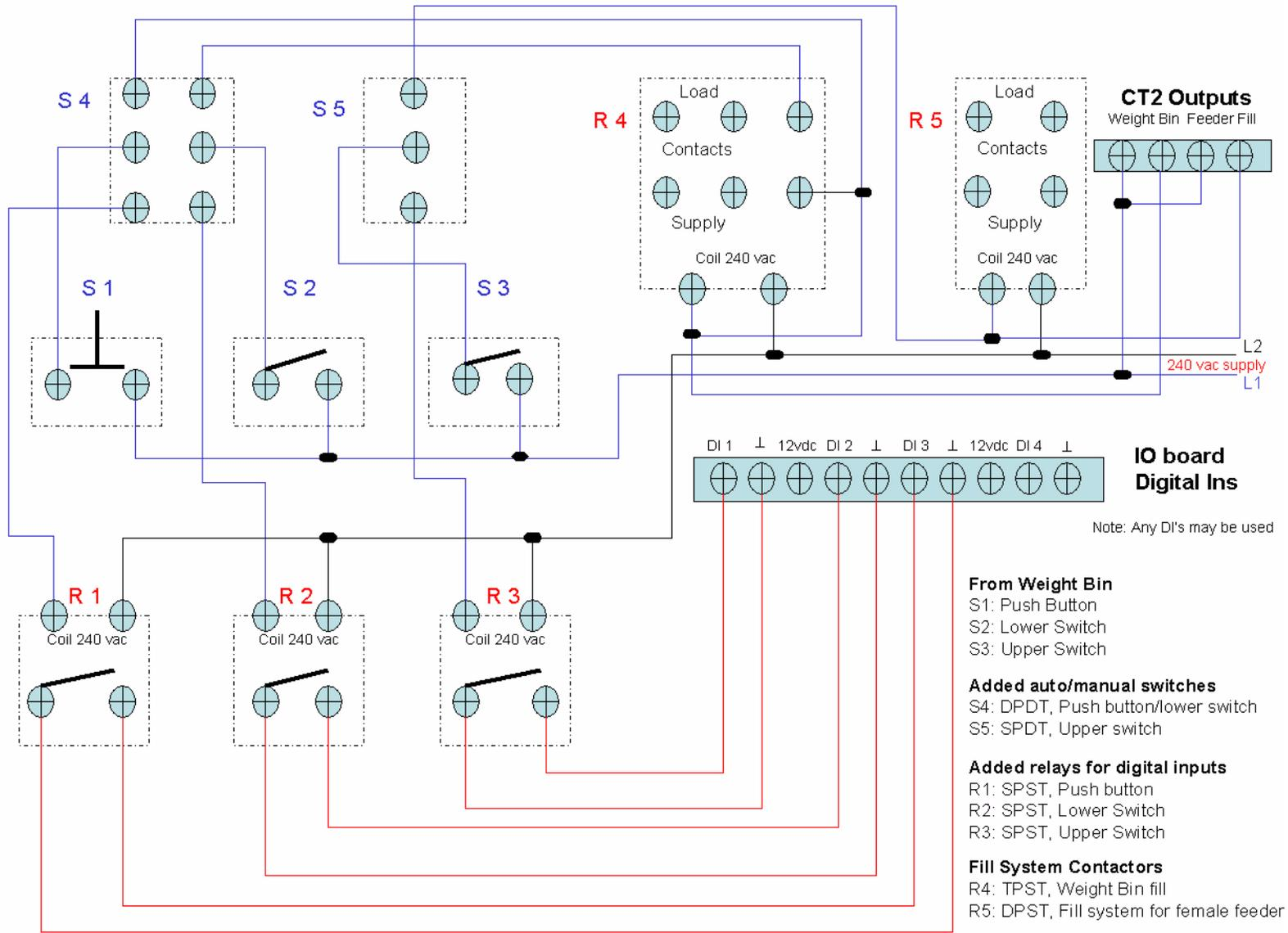
Figure 120. Weight Bin/Feeder Fill Wiring
