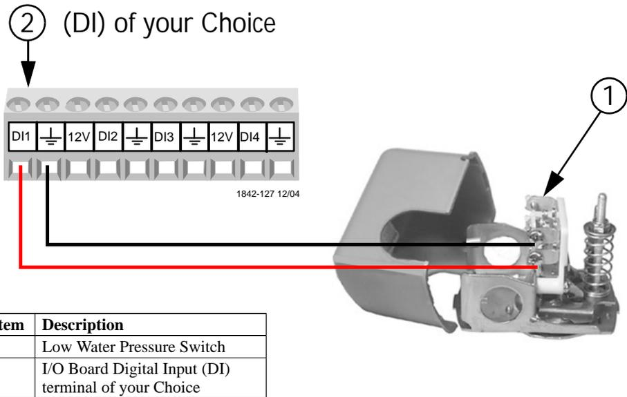
Figure 96. Low Water Pressure Switch Wiring
