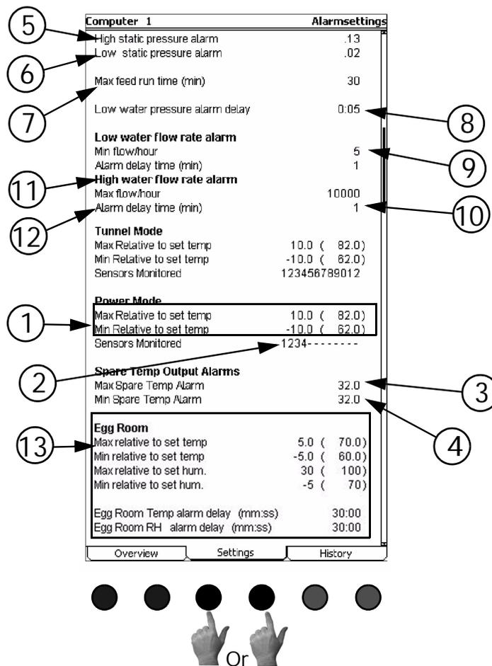
**Figure 41. Alarms Screen: Settings Tab**
