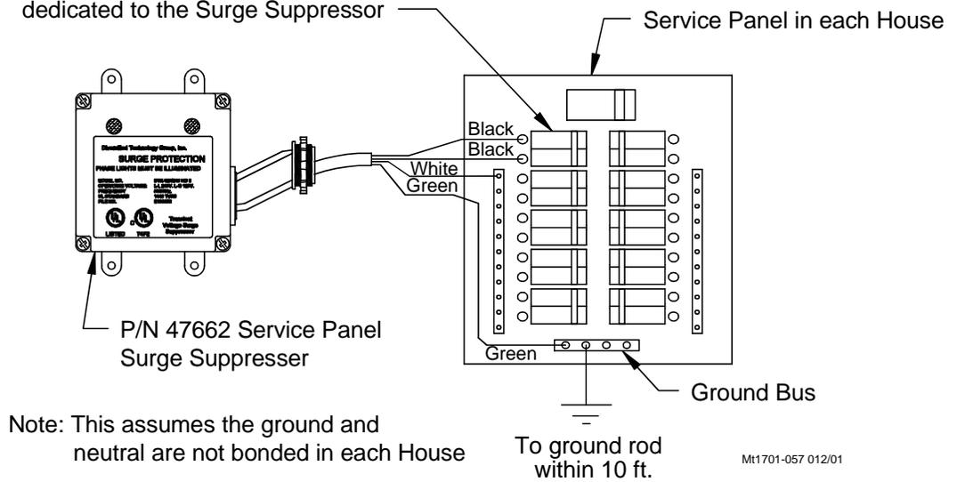
Figure 122. Main Service Panel Surge Suppressor Wiring
