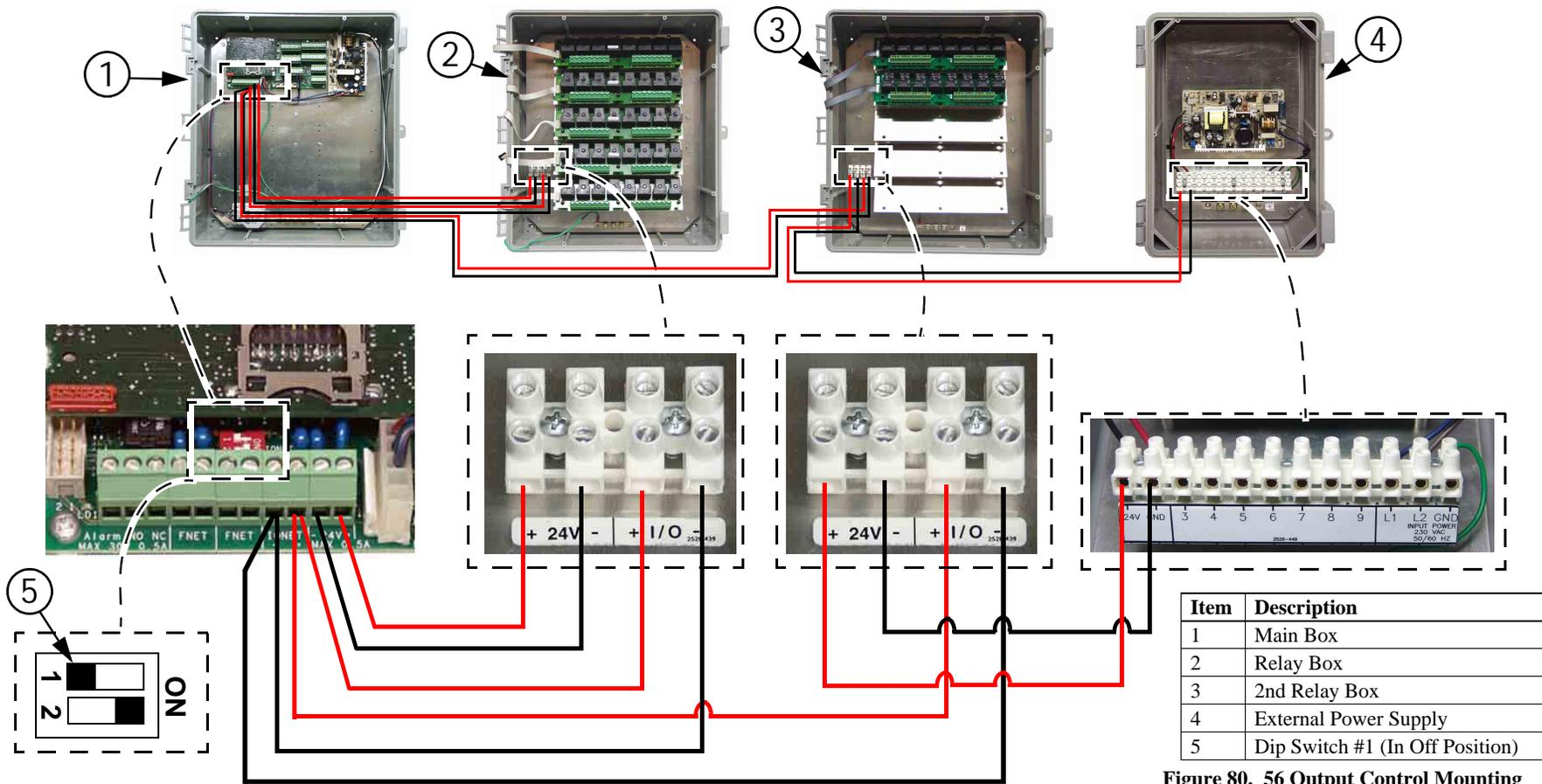
Figure 80. 56 Output Control Mounting
