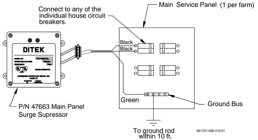
Figure 121. Service Panel Surge Suppressor Wiring
