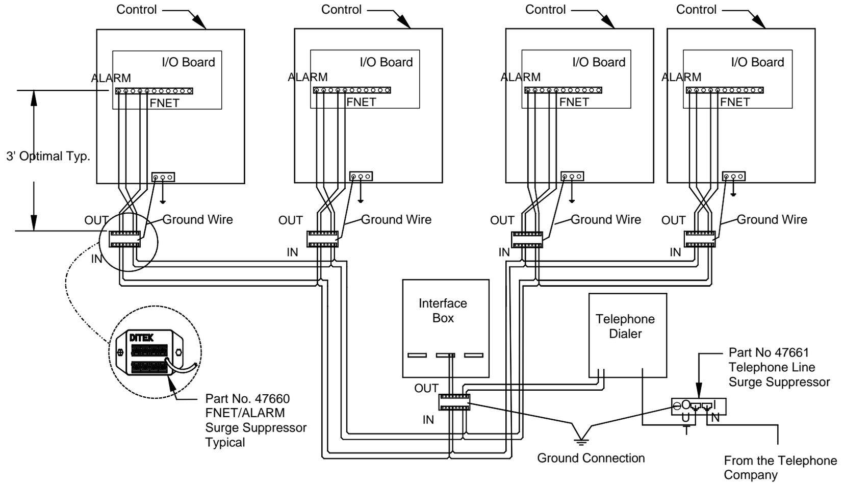
Note: There must be a ground rod within 10 ft. of the Ground Terminal of each Surge Suppressor. The wire size from the Suppressor to the ground rod should be 12 gauge or larger.
