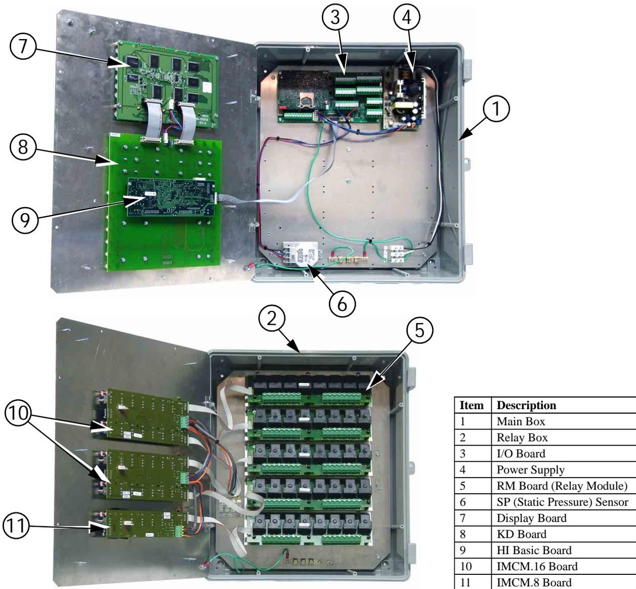
Figure 81. Wiring/Boards
