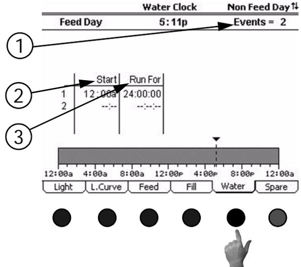
Figure 28. Clocks Screen: Water Tab
