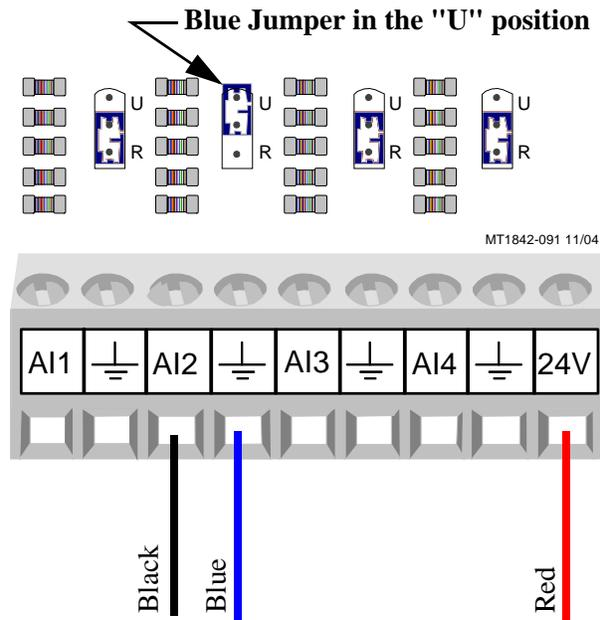
Figure 89. Static Pressure Sensor Wired to AI2
