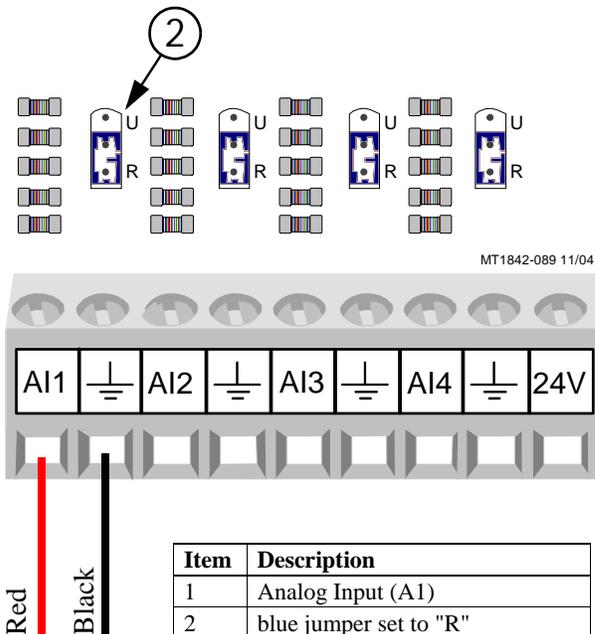
Figure 86. Temperature Sensor Wiring
