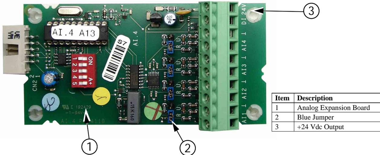
Figure 104. Analog Expansion Board
