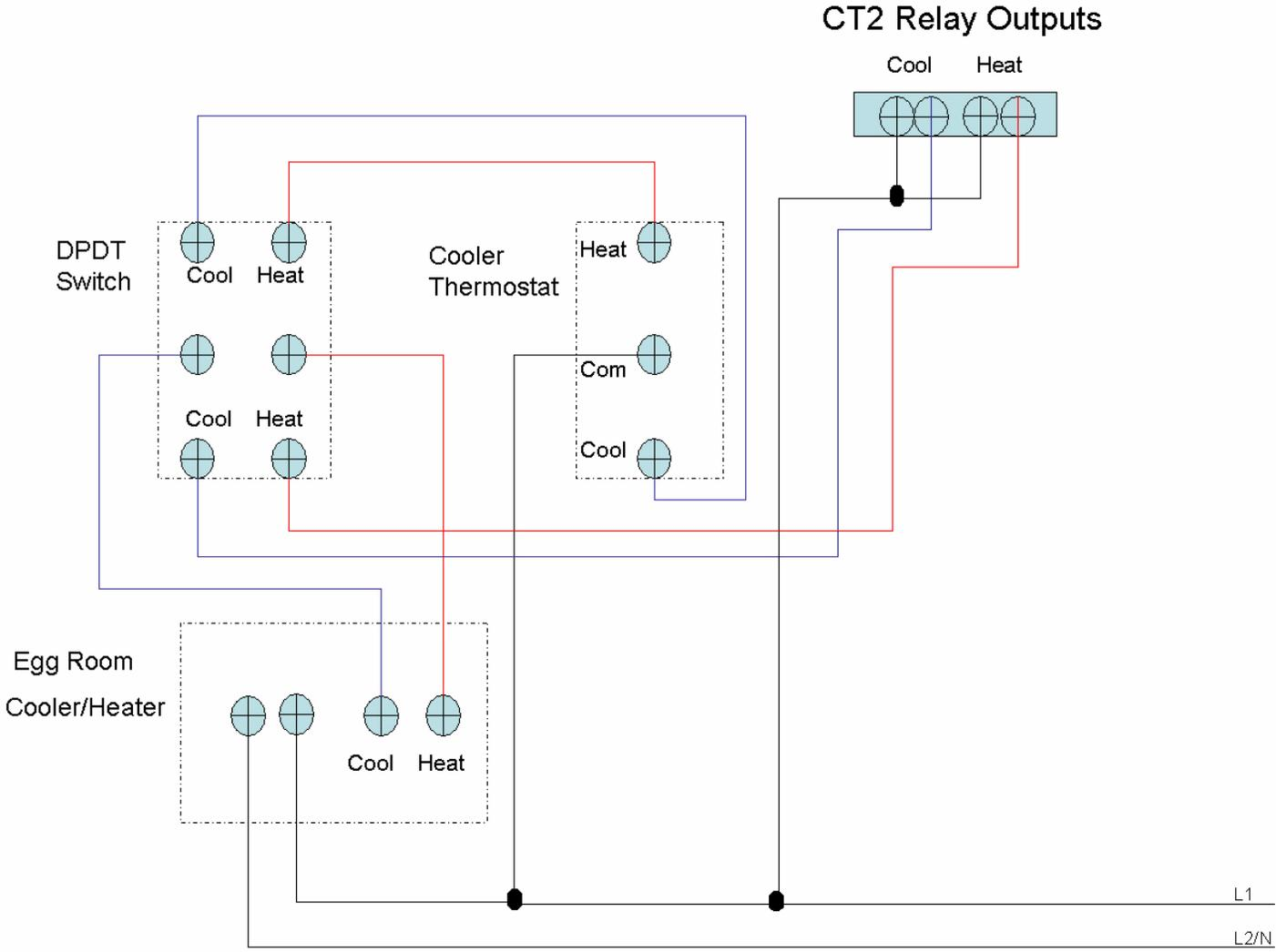
Figure 121. Backup Egg Room Cooler Wiring
