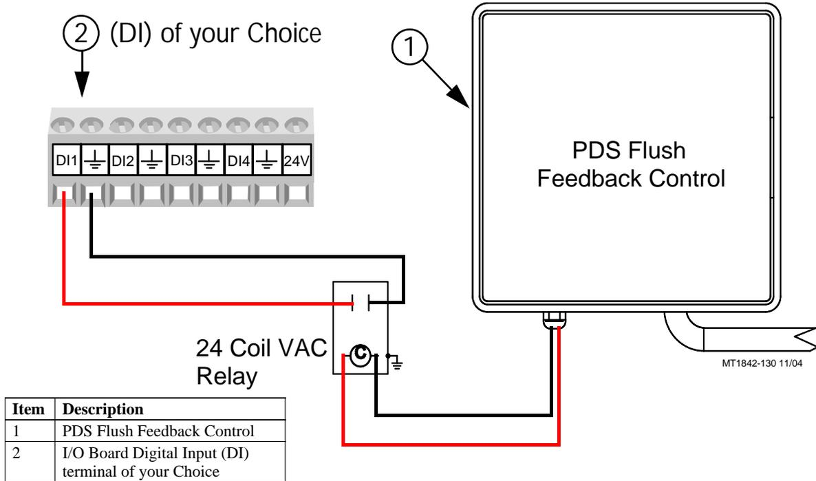
**Figure 100. PDS Flush Feedback Wiring**
