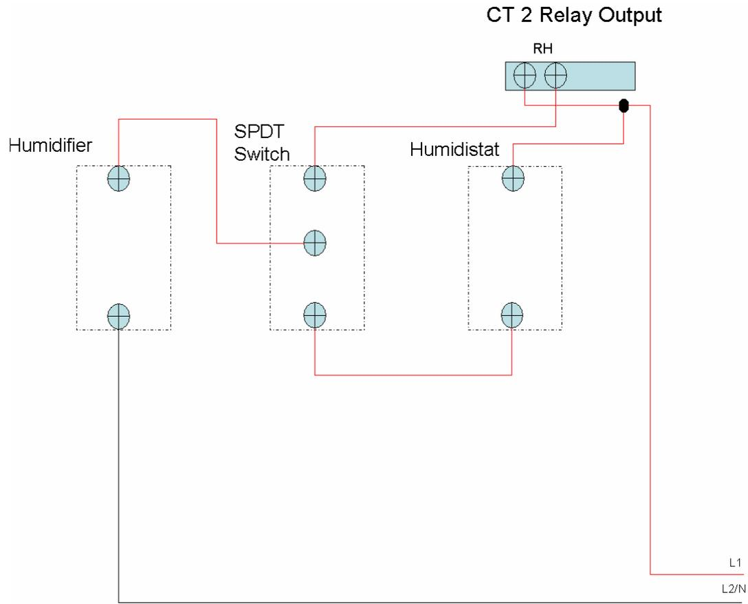
Figure 122. Backup Egg Room Humidifier Wiring
