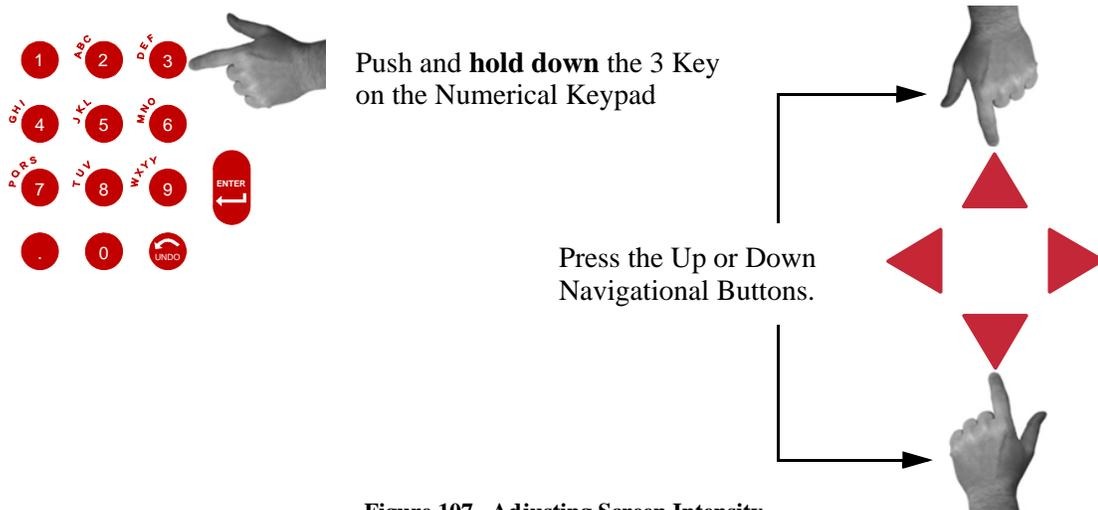
**Figure 107. Adjusting Screen Intensity**
