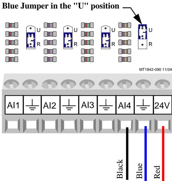
Figure 88. Static Pressure Sensor Pre-wired to AI4
