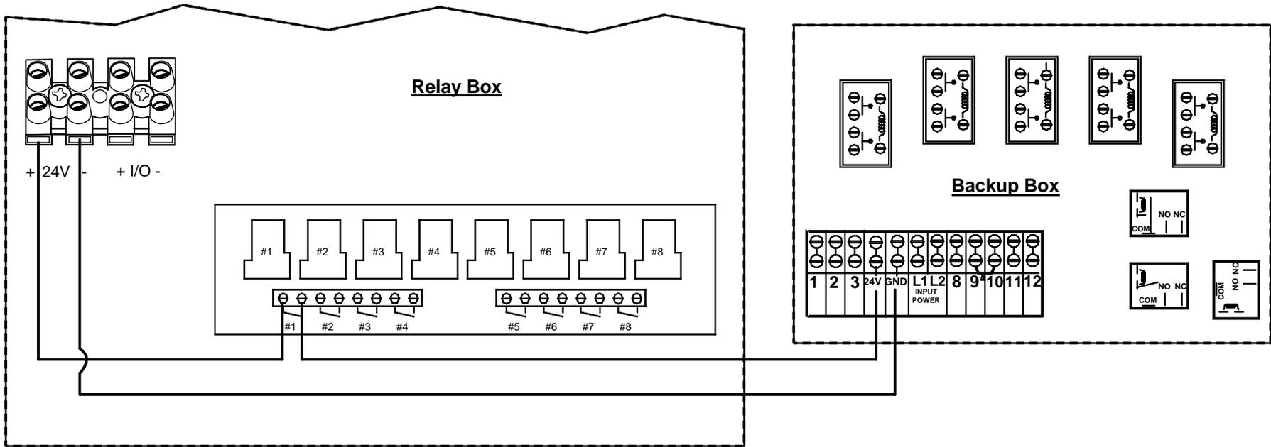
Figure 115. Backup Box Wiring
