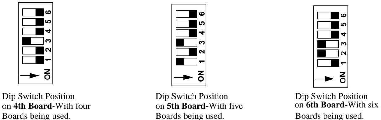
Figure 112. Dip Switch Settings 2nd Relay Box
