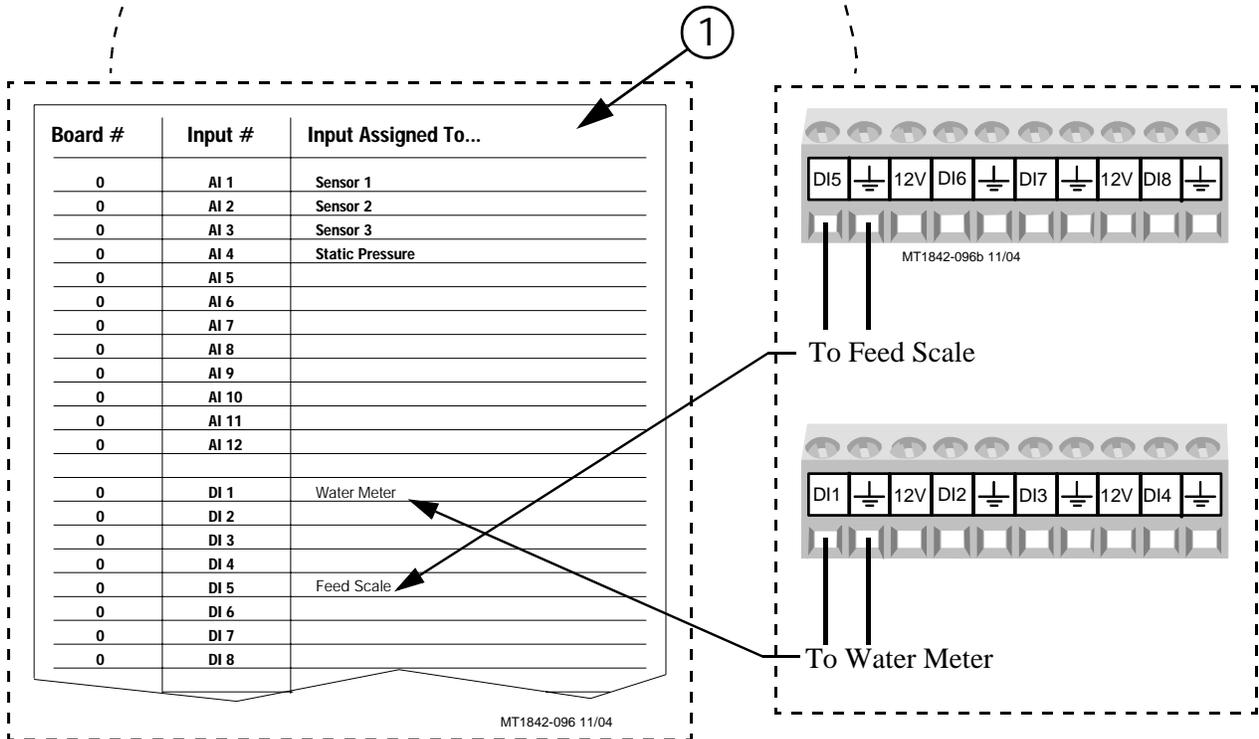
Figure 94. Digital Input Wiring
