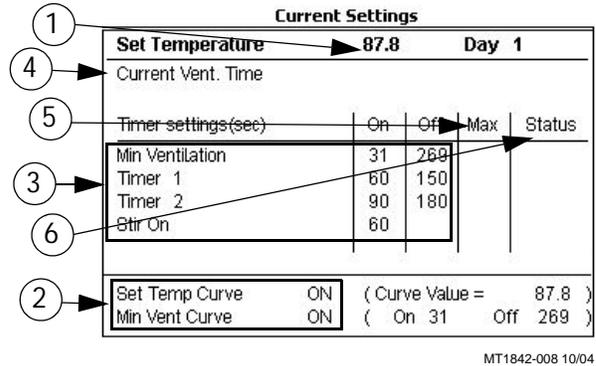
Figure 20. Screen 3: Set Temp/Min Timer
