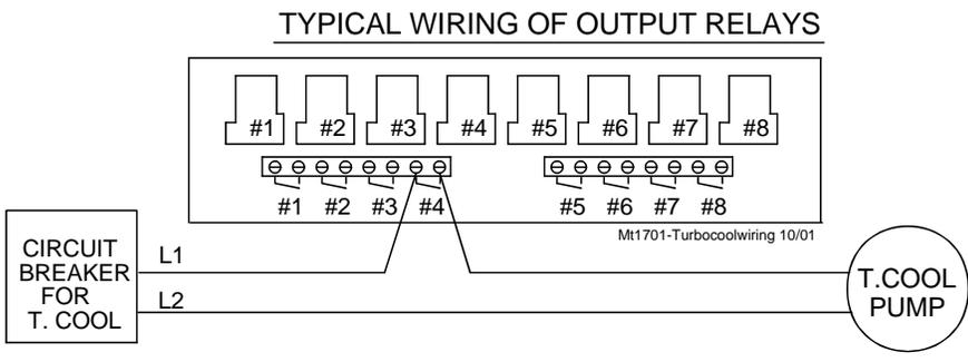
ALL OUTPUT RELAYS ARE SPST WITH DRY CONTACTS AS SHOWN. THIS SHOWS A TYPICAL SITUATION WHERE THE TURBO COOL PUMP HAS BEEN ASSIGNED TO RELAY 4 IN THE SETUP SCREEN.
