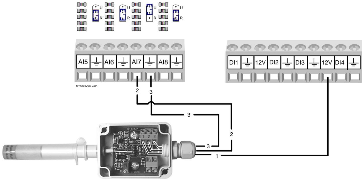
Figure 92. Relative Humidity Sensor Wiring
