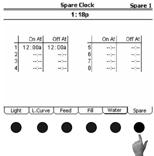
Figure 29. Clocks Screen: Spare Clock Tab
