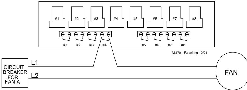
ALL OUTPUT RELAYS ARE SPST WITH DRY CONTACTS AS SHOWN. THIS SHOWS A TYPICAL SITUATION WHERE A FAN HAS BEEN ASSIGNED TO RELAY 4 IN THE SETUP SCREEN.
