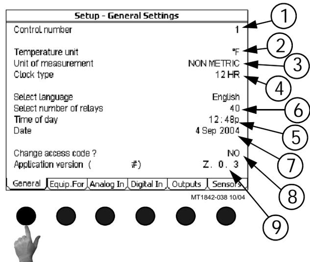
Figure 62. Setup-General Screen: General Tab
